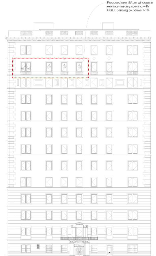
N2 NORTH ELEVATION - PROPOSED BUILDING ELEVATION 1/8" = 1'-0"
