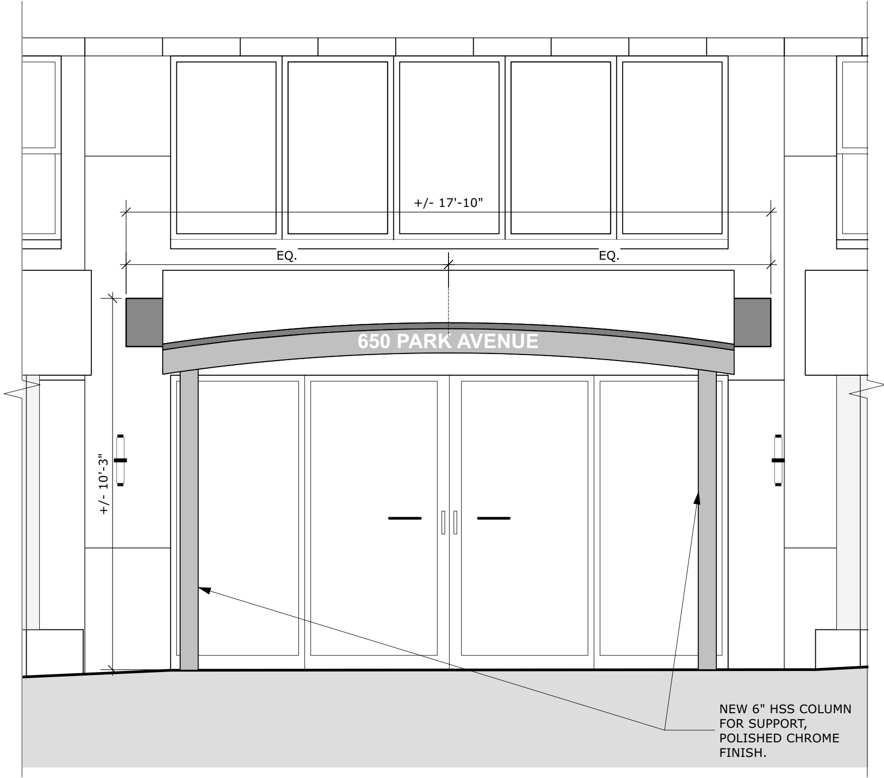
1 MAIN ENTRANCE ELEVATION - CANOPY Scale: 3/8" = 1'-0"
