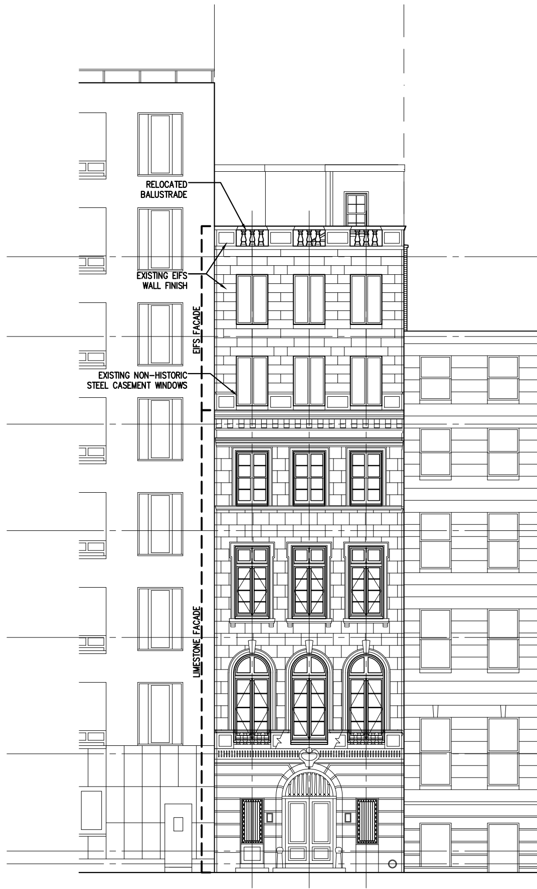
Existing Front & Side Elevations
