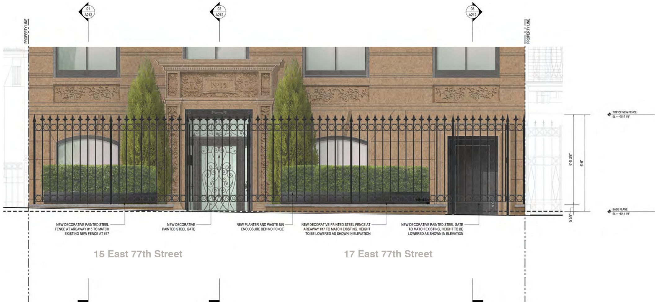
Areaway: Proposed Fence Elevation
