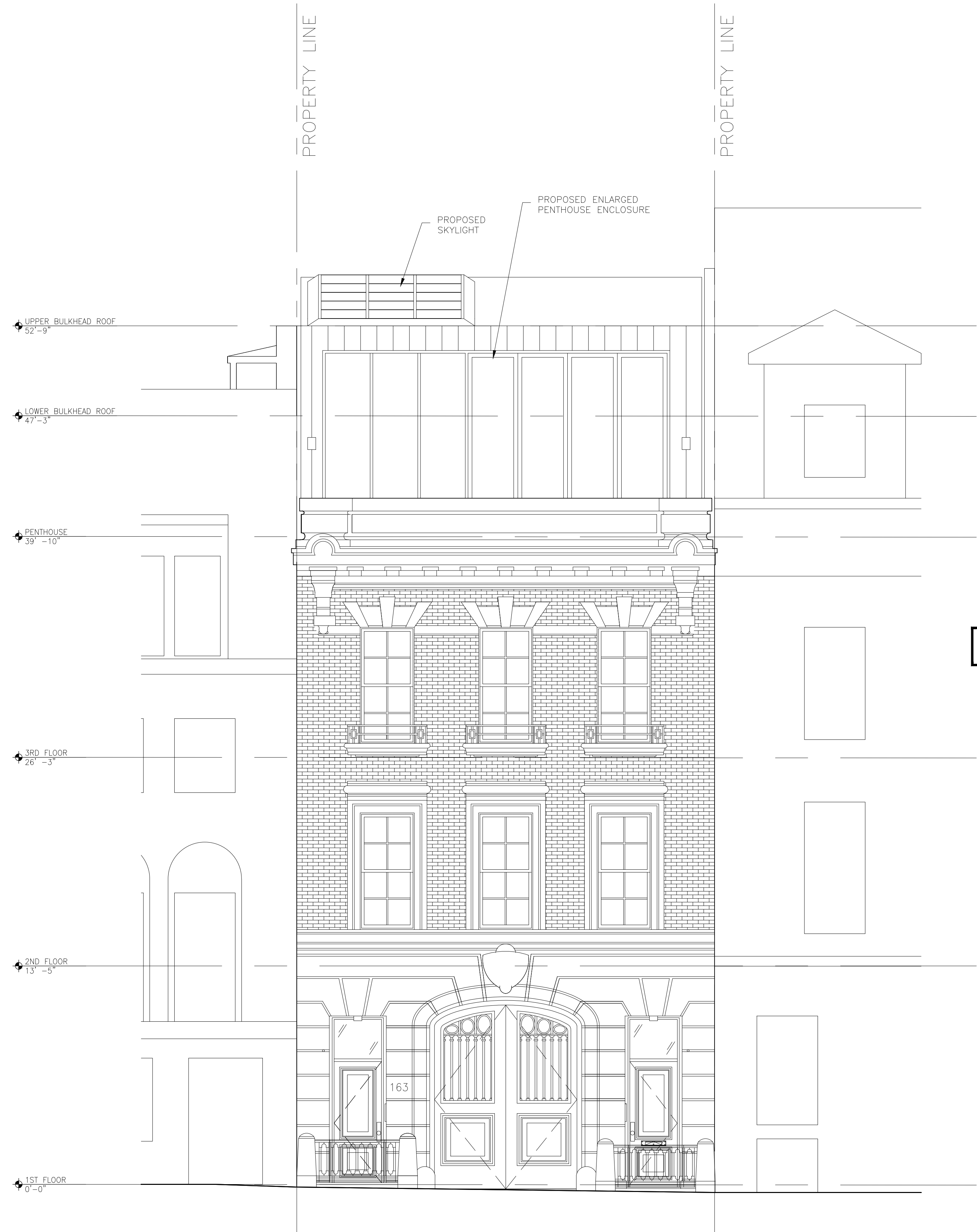
3 PROPOSED PENTHOUSE FRONT ELEVATION SCALE 1/4"=1'-0"
