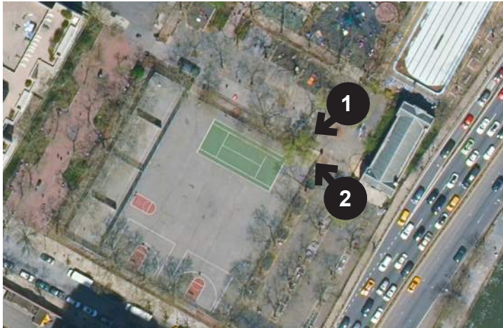
2 - Eastern Staircase to be replaced with new steps and ADA ramp. Drinking fountain out of contract limit and to remain.
