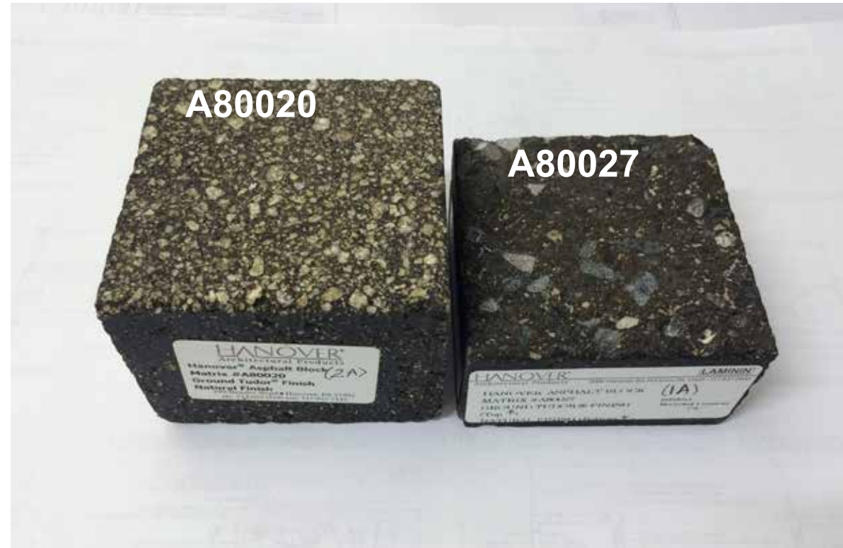
Asphalt block paver samples. Colors: A80020 & A80027. Finish: Ground tudor
