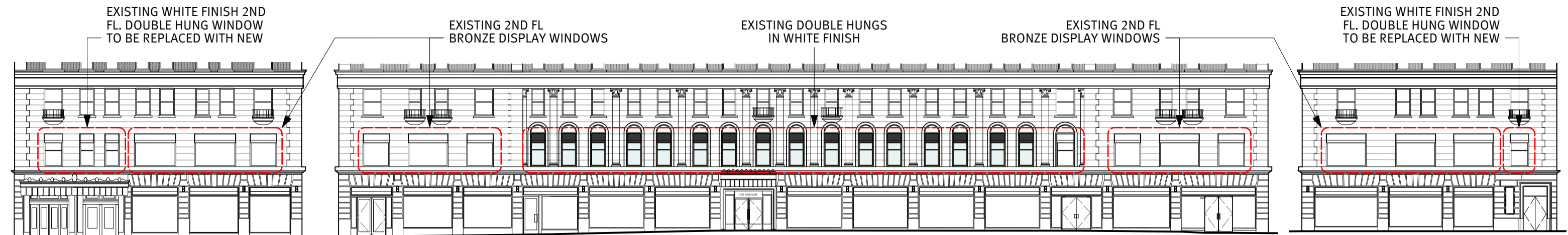
EXISTING SOUTH ELEVATION at E69th St.
