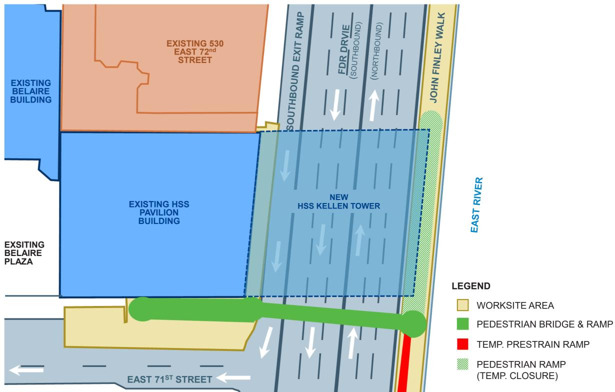
Notes: Diagram illustrative only | Subsequent site safety and logistics plans are being developed and will be approved for the building construction work
