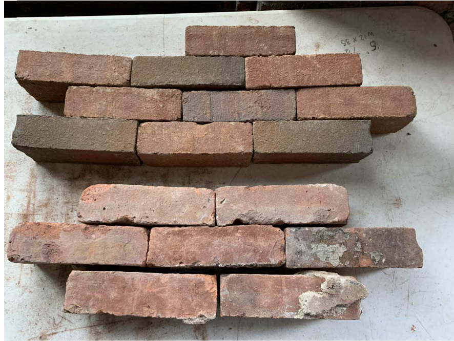
PHOTO SHOWS MIXTURE OF NEW (TOP) AND EXISTING SALVAGED (BOTTOM) BRICKS FOR COLOR COMPARISON.
