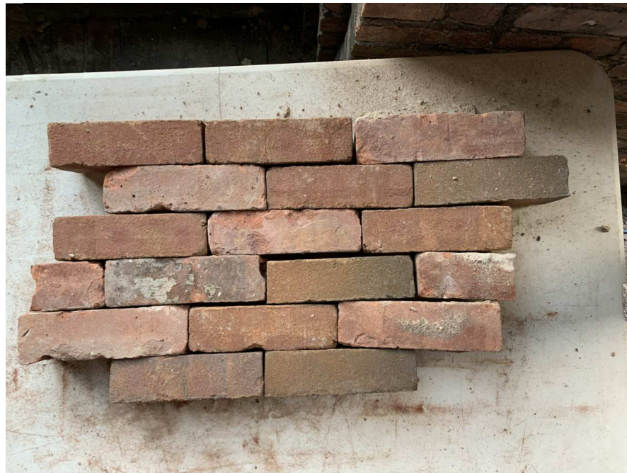
PHOTO SHOWS BLENDED MIX OF NEW AND EXISTING (SALVAGED) BRICKS PROPOSED FOR THE ELEVATOR BULKHEAD. NOTE: THIS WILL BE THE SAME BLENDED MIXTURE OF NEW AND SALVAGED BRICKS PREVIOUSLY APPROVED FOR PATCHING AND REPAIRS ON THE NORTH ELEVATION.
