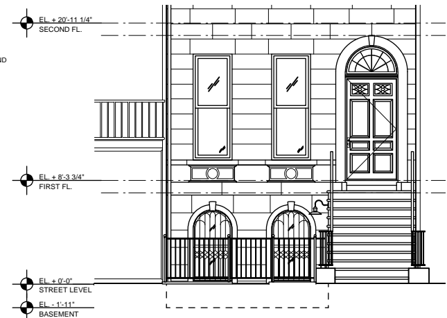
3) Existing North Elevation w/ Gate 3/32" = 1'-0"
