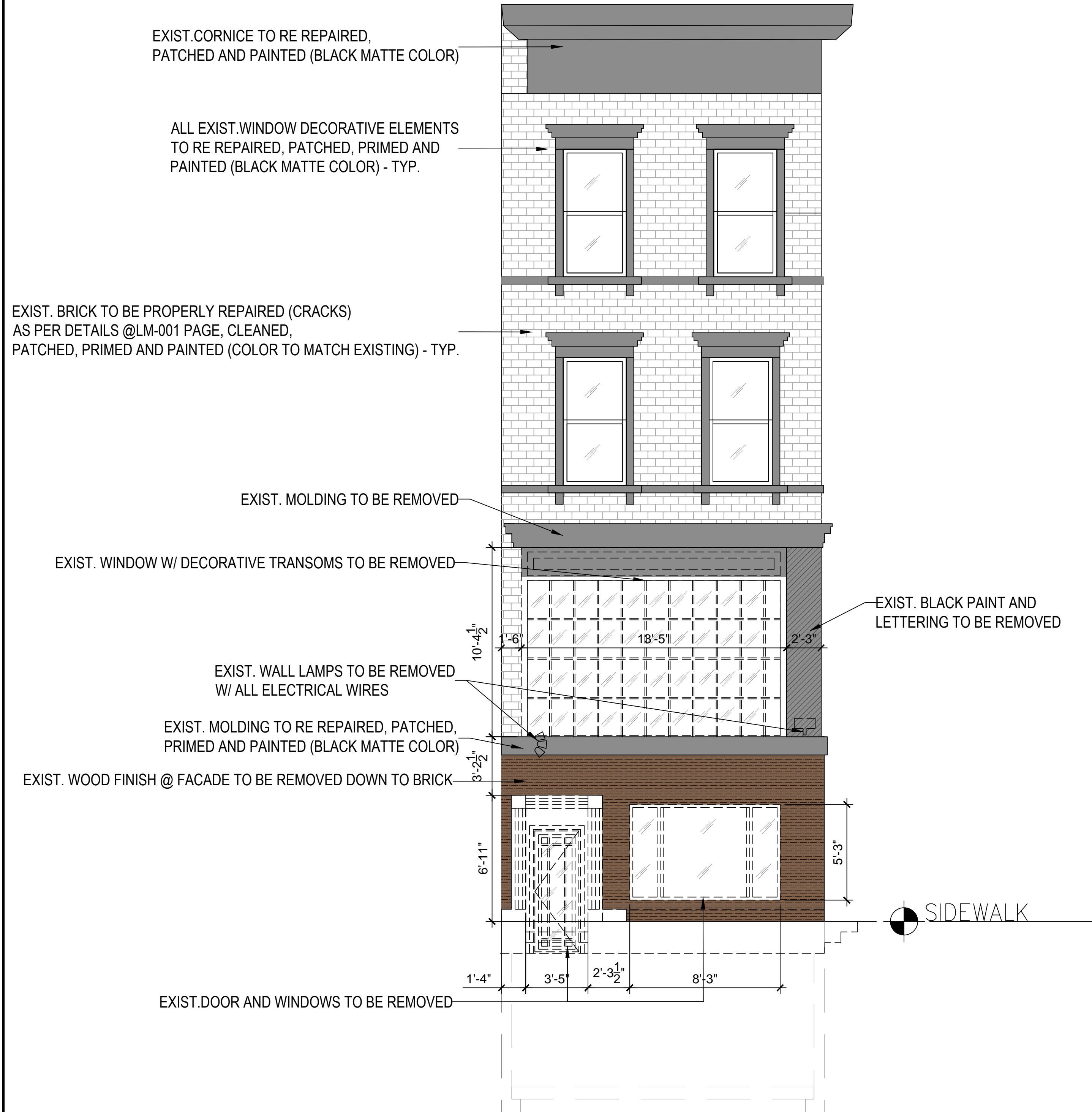
1 LEXINGTON AVENUE EAST ELEVATION - DEMOLITION SCALE: 1/4" = 1'-0"
