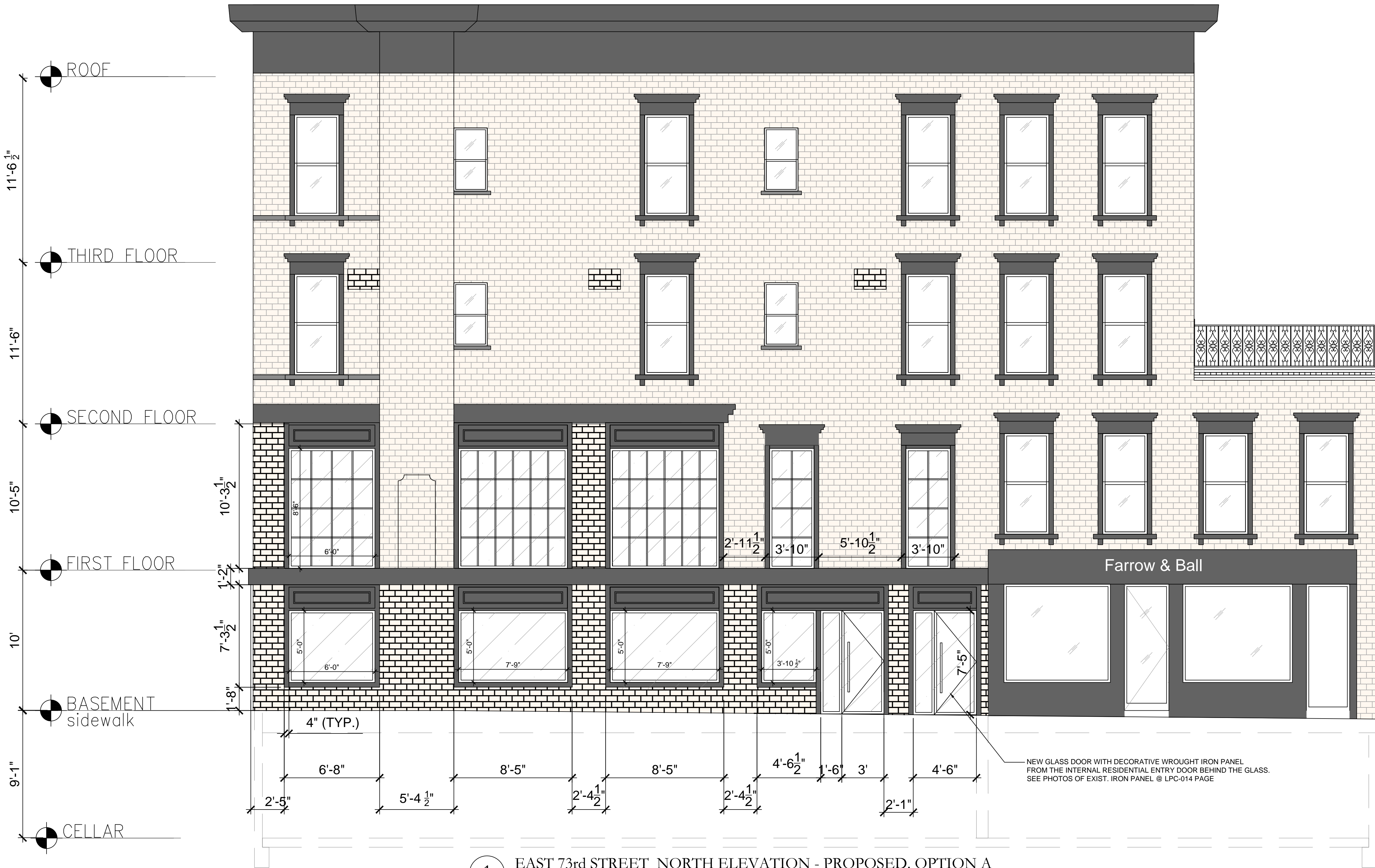
1 EAST 73rd STREET NORTH ELEVATION - PROPOSED. OPTION A SCALE: 1/4" = 1'-0"
