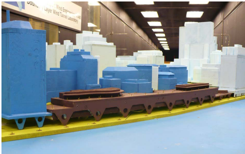
Figure 11: Wind Tunnel Test Model Views from South
