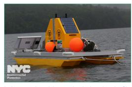
Last week, BWS Water Quality staff assembled and deployed a new robotic monitoring buoy on Neversink ervoir. The buoy is solar powered and it provides constant, near real-time monitoring data. This
