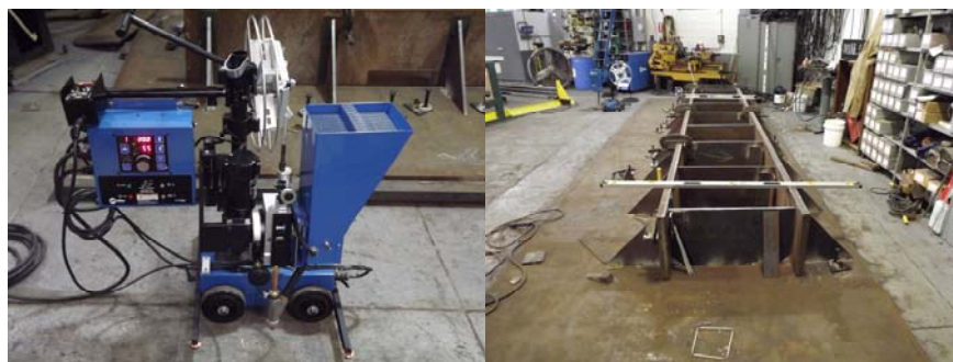
The Sub-Arc Welder Provides a Purer Weld With Less Contaminants From the Atmosphere. The Beam. (Credit: Thomas Whitehouse)
