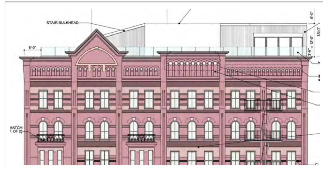
THE WINDERMERE BUILDING (2017) - THE GLASS RAILINGS WERE APPROVED BECAUSE THEY WERE NOT PERCEPTIBLE.
